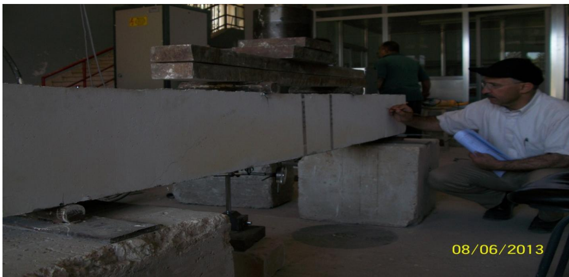
Figure 4: Experimental set up and crack monitoring
