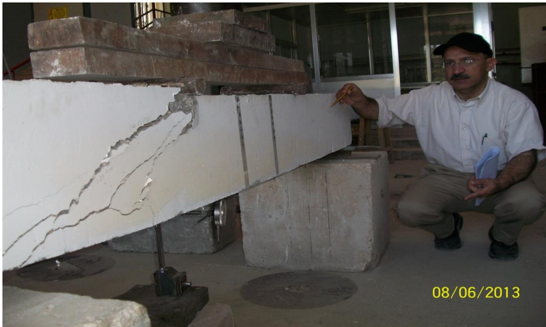
Figure 5: Beam BU at failure stage.
